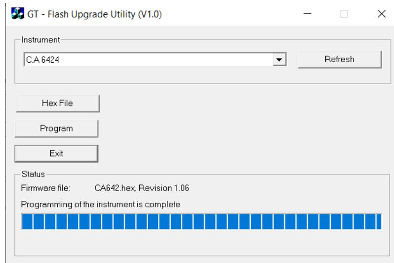
Once the download is complete, the utility will display “ Programming of the instrument is complete.
