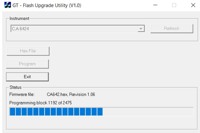
The download is progressing... On the device, the " TEST " button should be flashing, and the display should read " FLSH ".
