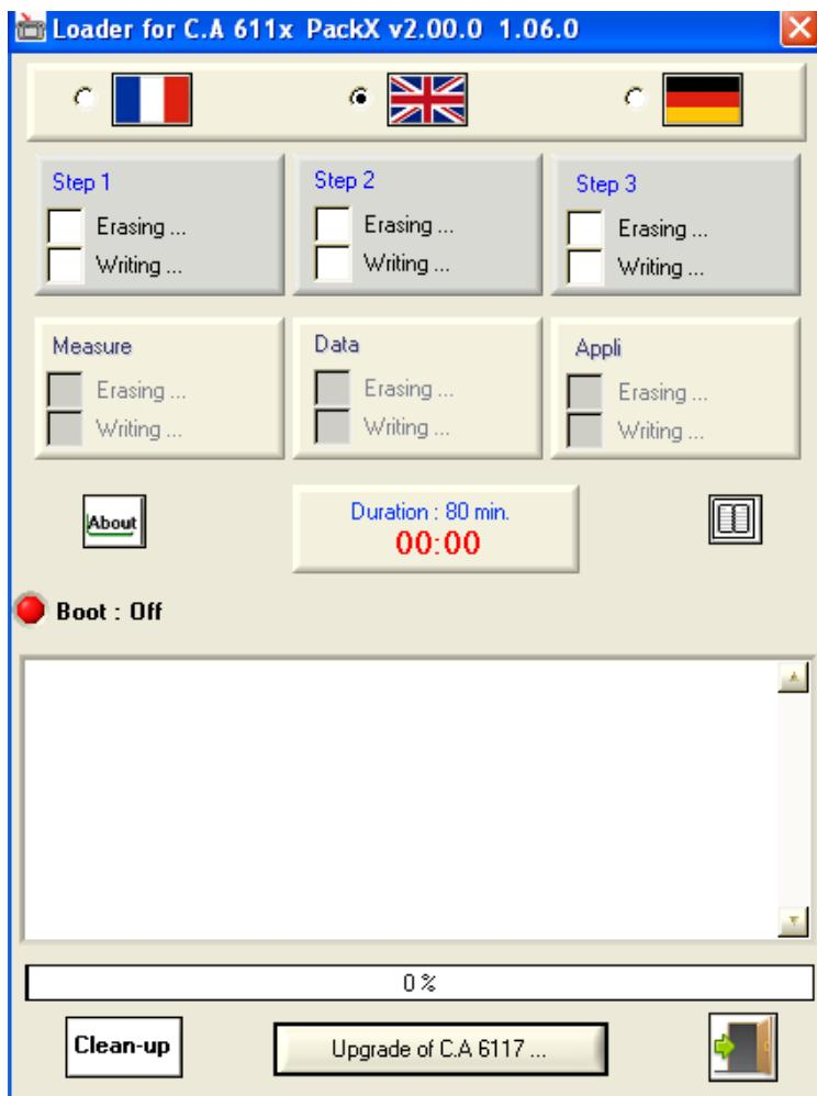
In order to upgrade the firmware on your C.A 611X instrument, click on the « Upgrade of C.A 611x... » button and strictly follow the procedure described in each pop-up window displayed by the program.
