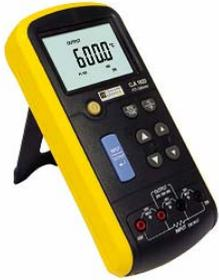
Want to calibrate your temperature sensors, resistive probes or process signals? To generate, simulate and measure all the low-level signals encountered in industry with a high degree of accuracy, Chauvin Arnoux is marketing a new range comprising 3 calibrators: the **C.A 1621, C.A 1623 and C.A 1631**.
