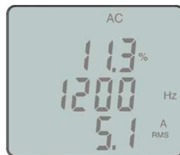
F407 SCREEN H3 harmonic measurement with a 400 Hz fundamental frequency
