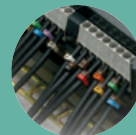
Simplified connection with screw-on terminal strip
