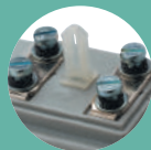
Split output terminals enabling risk-free short-circuiting of the secondary current (M4 or cage for 4 mm 2 wire)
