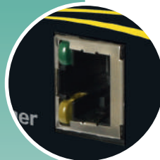
IEC 61850 server Ethernet port
