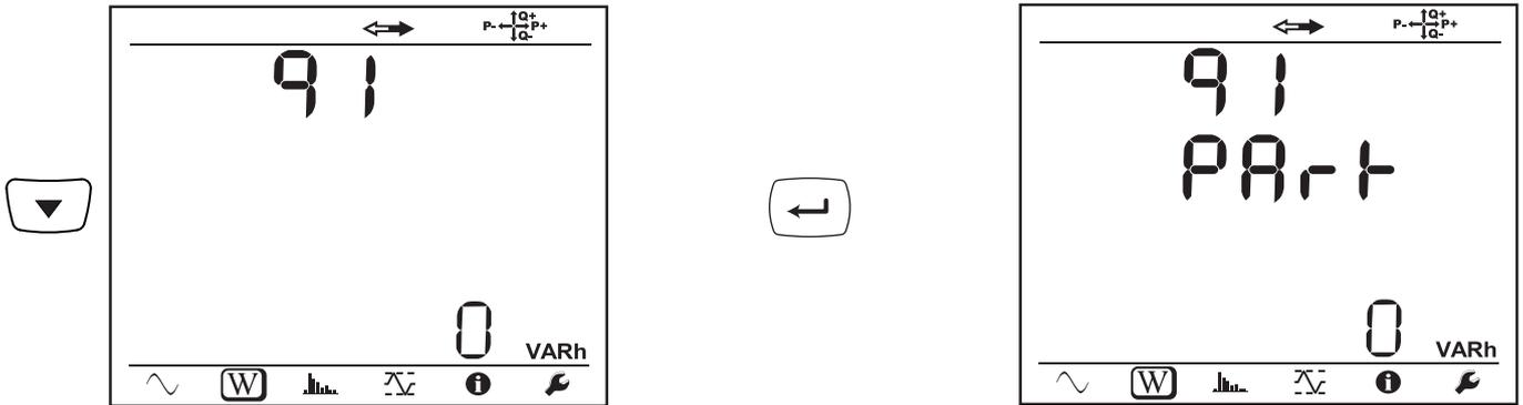
Eq2: Reactive energy delivered (by the source) in the capacitive quadrant (quadrant 2) in kvarh.
