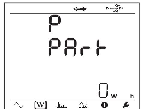
Ep-: Total active energy delivered (by the source) in kWh
