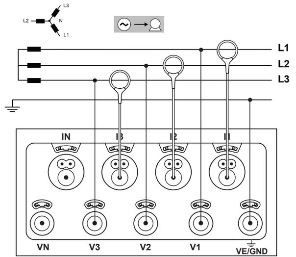
**4.1.3.7. Three-phase, 3-wire Δ balanced (with 1 current sensor): 3P-3W03**
