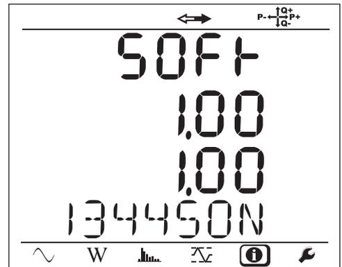
After 3 minutes with no action on the **Enter** or **Navigation** key, the display returns to the measurement screen
