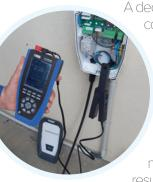
A dedicated function can be used to configure the transformation ratio of the current clamp, with current or voltage output (wide range of current clamps compatible with ASYC IV). Once this ratio has been defined, the multimeter directly displays the current value measured, making it easier to process the results.
