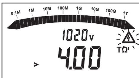
The insulation resistance is outside the measurement range.
