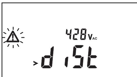
The spurious voltage present on the terminals is too high for a measurement to be made:
