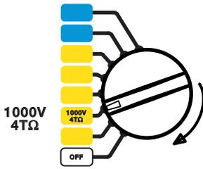
Start the measurement by a long press on the START/STOP key. The long press is acknowledged by an audible beep.
