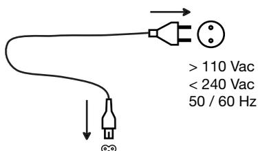
Connect the instrument to line power using the power cord.
