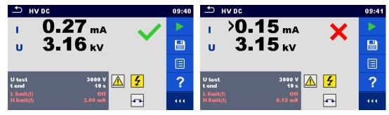
Figure 6.27: Examples of HV DC measurement results
