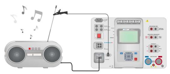
Figure 6.52: Measurement of Touch Leakage current
