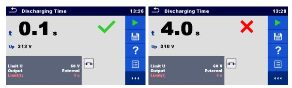
Figure 6.63: Examples of Discharging Time measurement results (Output = External)
