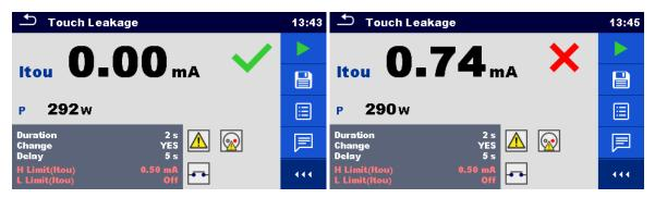
Figure 6.53: Examples of Touch Leakage measurement results
