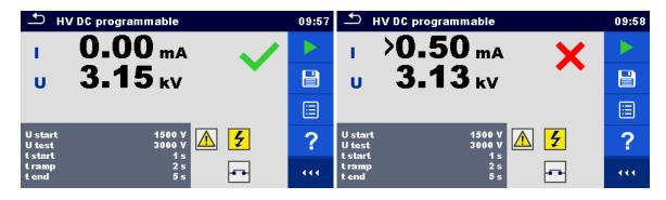
Figure 6.34: Examples of HV DC programmable test results
