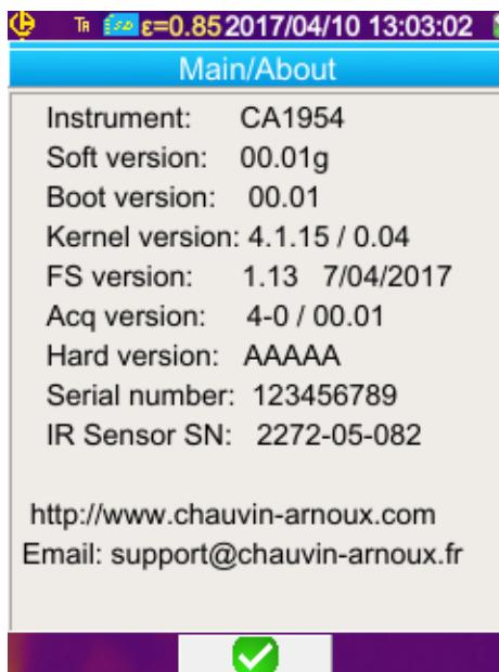
The current version of the camera's firmware is available from the "Main" menu by validating with **F2** → the item . The version number appears on the "Soft version:" line of this menu.
