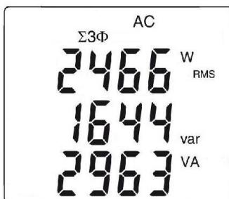
**Remark:** You can also measure the three-phase power on a balanced 4-wire network by proceeding in the same way, or by proceeding as for the measurement on a single-phase network, then multiplying the value found by three.
