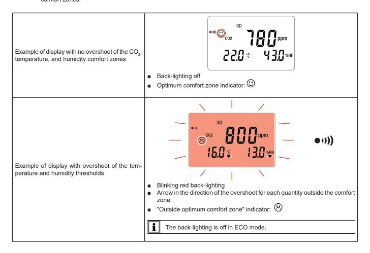
For the **1D** and **3D** modes, if the buzzer is active, it will sound intermittently upon the appearance of the  $\odot$  symbol.
