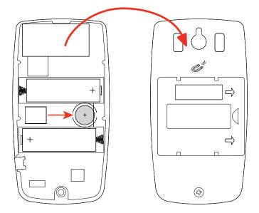
■ Remove the used button battery by lifting it and replace it with the new batter, respecting the polarity.
