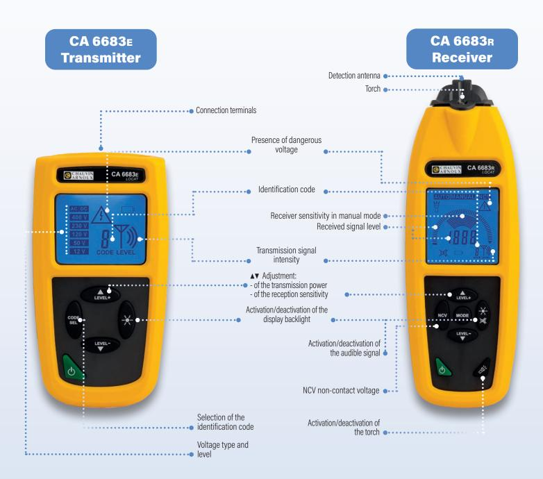
If voltage is present, the transmitter signals the danger and indicates its value.
