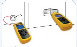
**Locate fuses**Connect the transmitter to a socket and simply find the corresponding fuse
