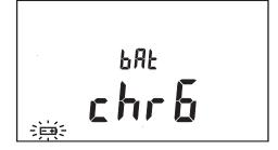
bAt on the small display and FULL in the main display means that charging is completed.
