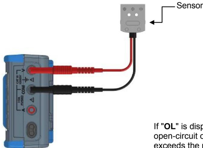
If "OL" is displayed, the sensor is open-circuit or the measured value exceeds the range limit.
