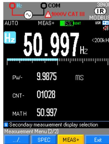
Depending on the triggering conditions of the frequency counter, calculation of the positive or negative pulses
