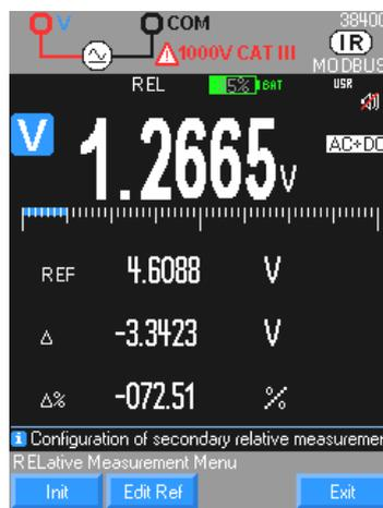
The main display unit and the horizontal bargraph track the evolution of the measurement at all times.
