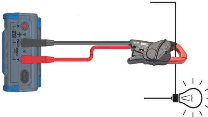
Current clamp with current output connected to the multimeter
