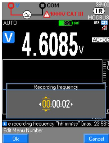
Validating **Freq.** by the [F3] key opens a menu for adjustment of the recording interval in hours, minutes, seconds
