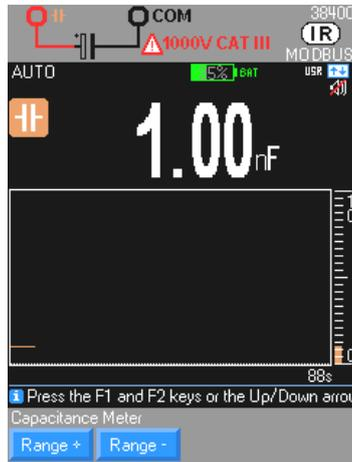
Measurement of the capacitance of a capacitor with a resolution of 1000pts
