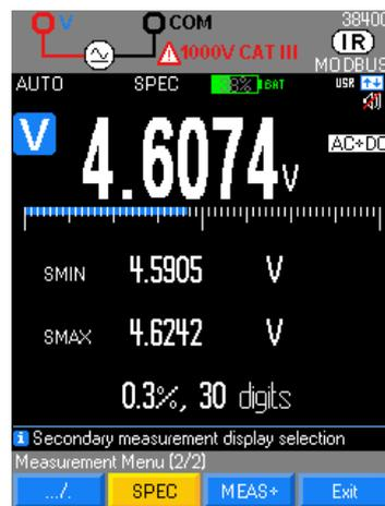
Using the internal technical specifications of the multimeter, the **SPEC** mode directly displays the tolerance on the measurement in progress, with no need to look for it and calculate it.
