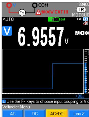
In this setting, the user can measure the true RMS value of an alternating voltage with its bias component (no capacitive coupling): "TRMS" measurement. In the "DC" mode, you measure a direct voltage or the DC component of an AC voltage.
