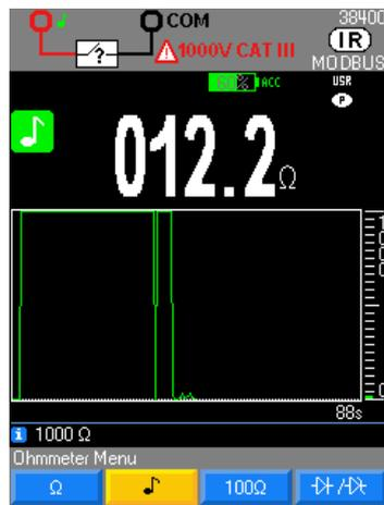
Measurement of a resistance up to 1000Ω, with continuous 4kHz audible indication.
