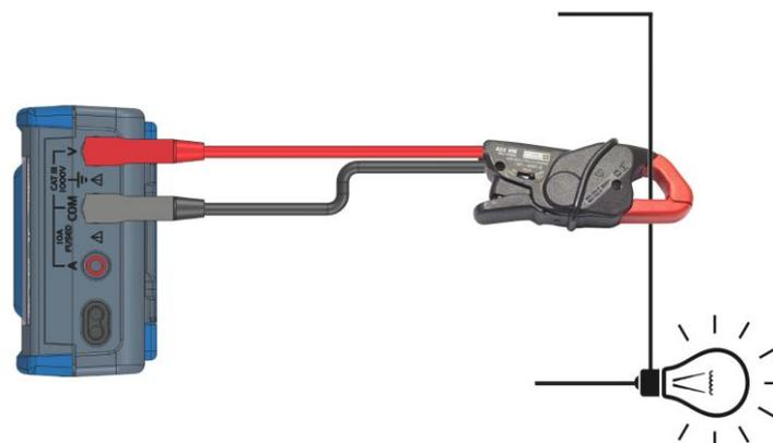
Current clamp with voltage output connected to the multimeter
