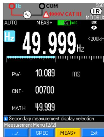
Depending on the triggering conditions of the frequency counter, measurement of the pulse width in ms.
