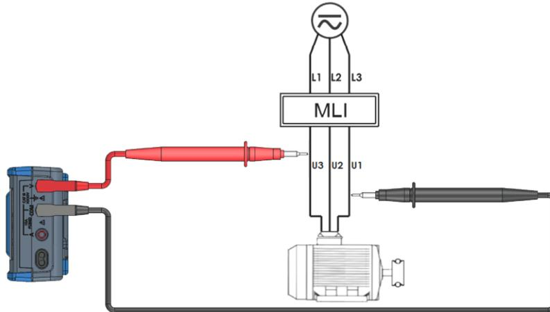
Connecting the multimeter to filter a current >300Hz
