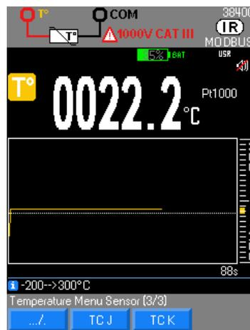
Measurement of the temperature with a sensor: Pt100/Pt1000 or ./...
