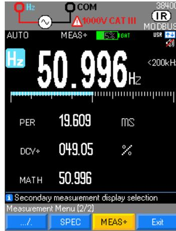
The DCY duty cycle mode is optimized to measure the active or inactive intervals of switching signals or logical signals. Electronic fuel injection systems and switching power supplies, in particular, are controlled by pulses of variable width that can be verified by a duty cycle measurement.
