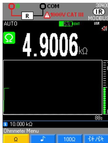
In the  $50\text{ M}\Omega$  range, in order to avoid the influence of the mains and guarantee the stated specifications, it is best to disconnect the multimeter from the Wall Plug.
