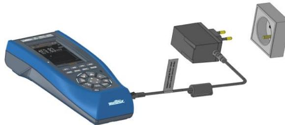
You can charge the storage batteries without removing them. Use the external charger supplied with the multimeter. During the charging, the multimeter remains operational.
