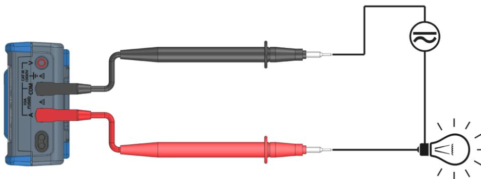
3. Read the measurement indicated on the main display unit.
