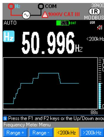
Select the Hz function to measure the frequency of the voltage
