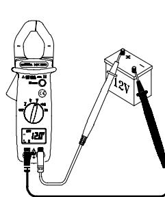
Set the switch to V ==. Connect the red test lead to the "+" input terminal and the black test lead to the "COM" input terminal. Then place the touch prods in contact with the points where the DC voltage is to be measured. Then read the result on the display.
