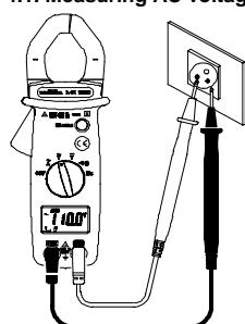
Set the switch to V~. Connect the red test lead to the "+" input terminal and the black test lead to the "COM" input terminal. Then place the touch prods in contact with the points where the AC voltage is to be measured. Then read the result on the display.
