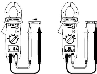
**4.7. Measurement of the voltage frequency
