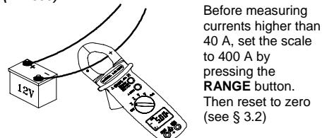
Open the jaws of the clamp by pressing the trigger and insert the cable to be measured between them. Close the clamp and read the result of the measurement on the display.
