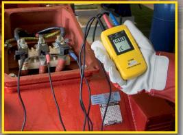
The C.A 6608 and C.A 6609 are essential instruments for identifying the order of the phases on an electrical installation and the rotation direction of any industrial equipment connected to the installation. Comprehensive and easy to use thanks to the colour-coding of the terminals and cables, these instrument are ideal for industrial building verification and maintenance teams.
