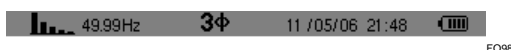
Figure 18: The 3 \phi sign at the top of the screen indicates a balanced three-phase connection configuration.
