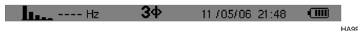
Figure 35: The 3 \phi sign at the top of the screen indicates a three-phase configuration.
