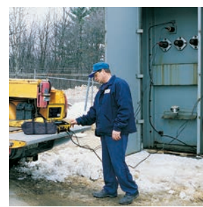
Measurement on a 2,000 kVA three-phase transformer in the field
