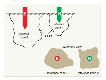
As diffusion of an electric current depends on the soil resistivity, it is difficult to be sure that the zones of influence have been avoided. The best way of confirming the measurement is therefore to repeat it after moving the stake S so that you can make sure it is similar to the earlier measurement.
