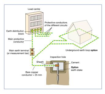
Whatever the type of earth electrode chosen, its purpose is to remain in close contact with the soil so that it can provide a connection with the earth to drain any leakage currents. The quality of an earth electrode depends on three key characteristics:
