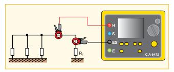
Instead of a single clamp containing the generator circuit and the receiver circuit, two clamps are used, with one serving as the generator and the other as the receiver. The advantage of having one clamp per function is that you can perform measurements on conductors where the earth clamp is not suitable, because of its clamping capacity or its thickness.
