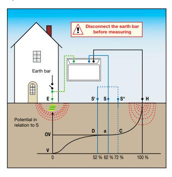
Example: Measurements at different distances R1 to R9 from 10 to 90 % of the distance SH
