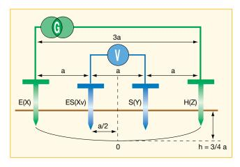
Note: the terms X, Xv, Y and Z correspond to the former naming conventions used for the E, Es, S and H electrodes, respectively.
