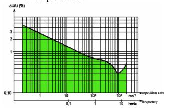
In this curve (50 Hz network) , the acceptable measurement point should be located in the green area.
