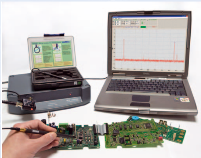
Below: use of the contact probe and use of the amplifier connected directly to the MTX 1050.
