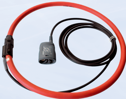
HX0072 AmpFLEX™ current sensor 5 A - 3 000 Arms / 200 kHz
