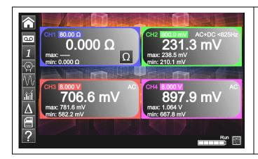
Channel 1 of the **ScopiX** is named CH1. It is used to measure various physical quantities in addition to the signal amplitude measurements, using the appropriate **Probix** accessories. The other channels are voltmeter channels only (or current channels, when used with a **Probix** clamp).
