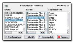
Selection of more than 10,000 manufacturer references stored in the database inside the instrument. It is a simple task to update this list, either directly on the instrument by means of its touch screen, or in your office with the management software delivered with the FTV200.
