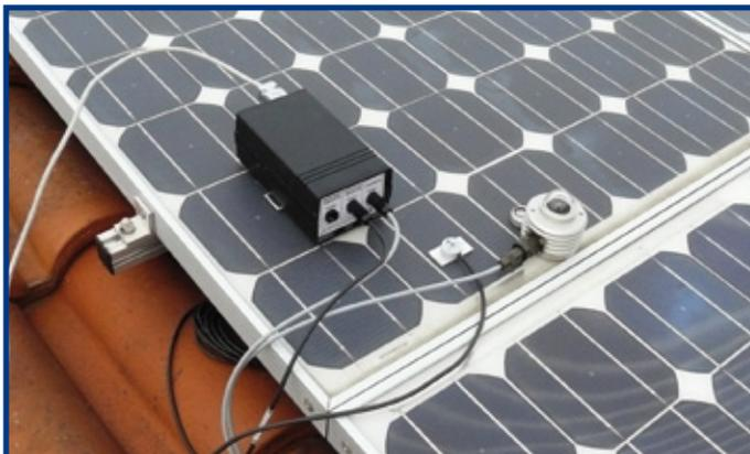
The **GREENTEST** comes with a set of communication accessories which are particularly useful for transmitting measurement results on large installations. A «REMOTE» module allows real-time data transmission up to 100 m away.
